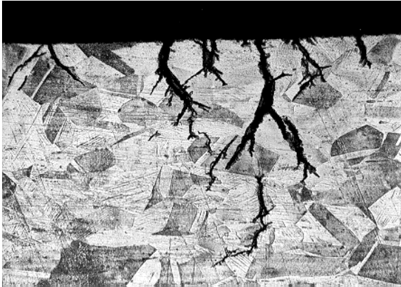
Figure 2. Stress corrosion cracks in stainless steel in dilute wash water.
