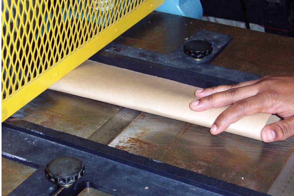
Figure 2. Typical loosely folded sample being sent through the Honshu tester nip.
